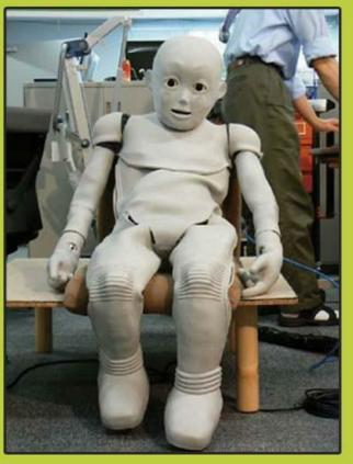
The CB2 (the "Child Robot") is another project developed by the researchers at Osaka University. CB2 has the physical and intellectual abilities of a 2-year old. It was built with cameras for sight, microphone, and tactile sensors to simulate a sense of touch and feeling. "One day," says Professor Ishiguro, "they will live among us. Then you'd have to ask me, "Are you human?"
