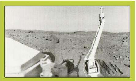
On February 12 and 13, 1977, Viking Lander I dug a series of deep trenches on Mars to provide samples, from as far as 30 centimeters (12 inches) below the surface. This is the actual view from the robot craft.
