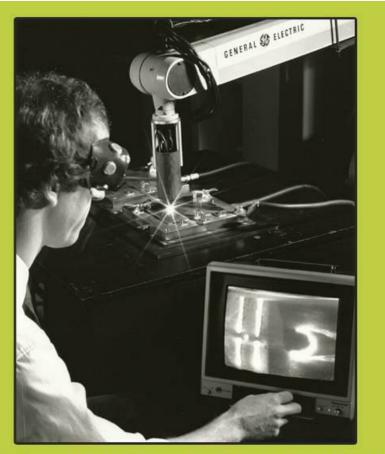
This General Electric robot has a sensor system that brings the powers of sight and intelligence to welding robots. The advanced vision and control system enables a welding robot to steer itself along irregularly shaped joints, continually observing the joint and weld "puddle" and making adjustments as it travels along.
