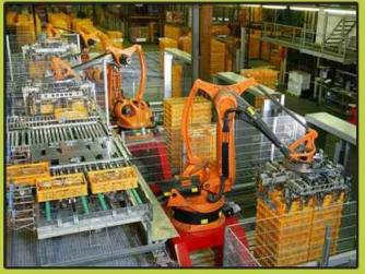
Modern robot packers at work packing bread.
